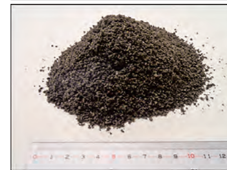
Molten slag MS5 (fine aggregate)
